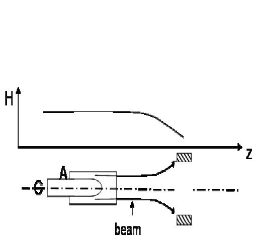
Fig. 4. Scheme of irradiation of the inner cylindrical surface of samples in the decreasing magnetic field
