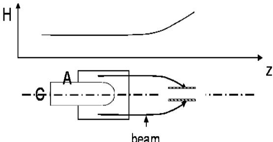
Fig. 6. Scheme of irradiation of the outer cylindrical surface of samples in the increasing magnetic field.
