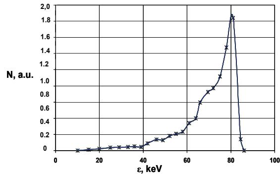
Fig.2. The energy spectrum of the electron beam of the accelerator
