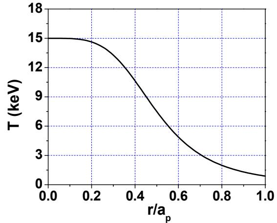
Fig.4. Typical temperature profile for the HELIAS stellarator with five periods of magnetic field.
