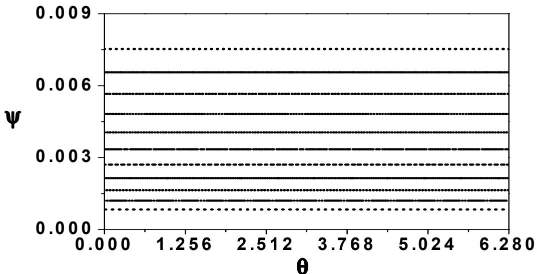
Fig.1. Vertical cross- section of the magnetic field configuration in the toroidal system without island chains in flux coordinates (Magnetic induction flux  $\Psi$  through the magnetic surface versus the poloidal angle  $\theta$ ).
