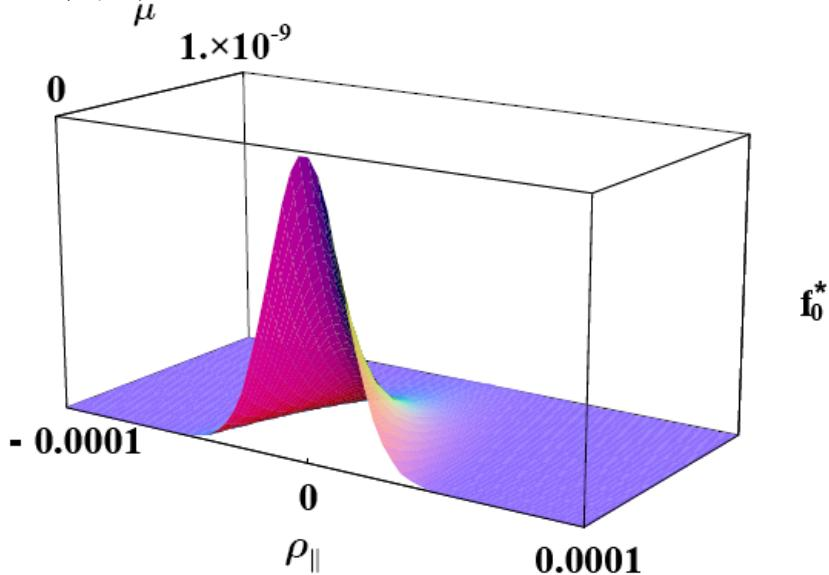
Fig.5. Maxwell guiding center distribution function  $(\mu, \rho_{||})$ .
