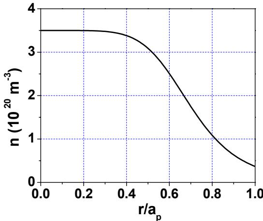
Fig.3. Typical density profile for the HELIAS stellarator with five periods of the magnetic field.
