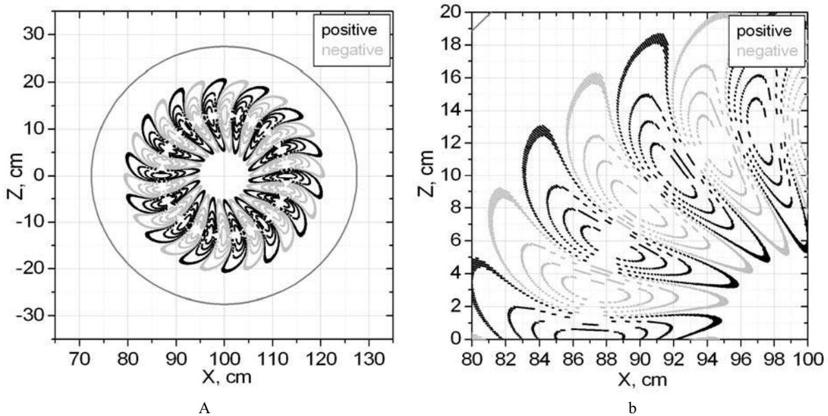
Fig. 2. Vertical cross-section of the electric field potential (equipotential lines), a – general view, b – enlarged section.
