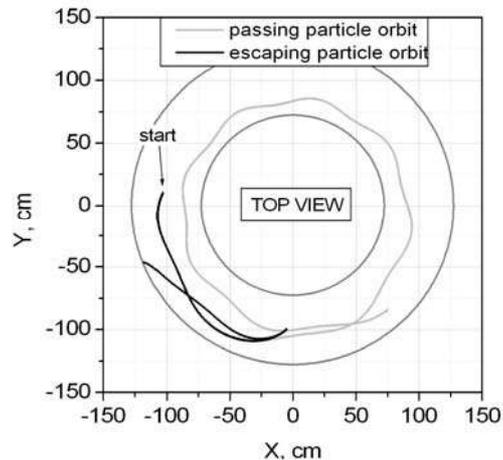
Fig. 10. Top view of the passing (grey) and escaping (black) test particle orbits.
