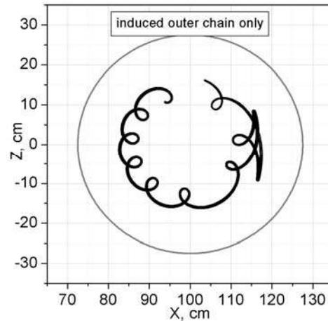
Fig. 12. Test particle orbit under the potential  $\Phi_2(r-r_{02})$  taken separately.  $\omega^* = 1.61 \cdot 10^7 \text{ sec}^{-1}$ .
