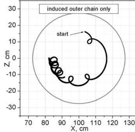
Fig. 8. Test particle orbit under the potential  $\Phi_2(r - r_{02})$  taken separately.
