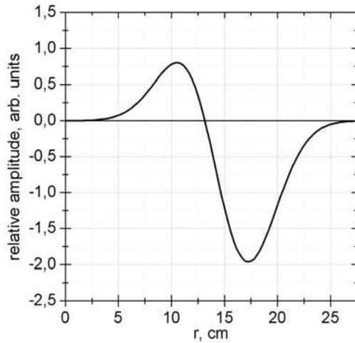
Fig. 3. Radial distribution of the electric field potential
