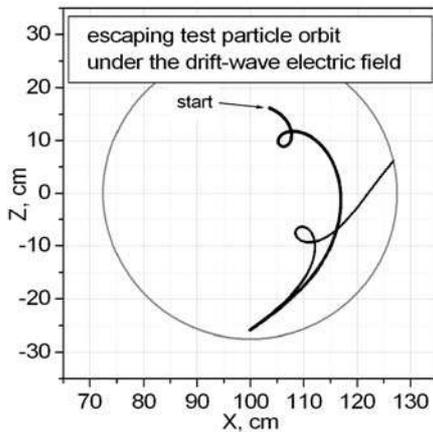
Fig. 9. Effect of two drift-wave potentials on the test particle orbit.
